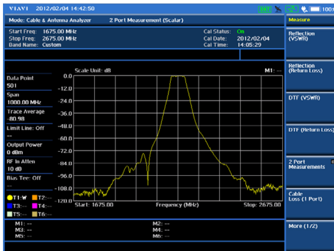
Cable and antenna test — 2-port Measurement
