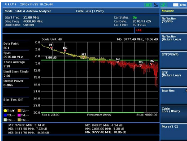
Cable and antenna test — Cable Loss
