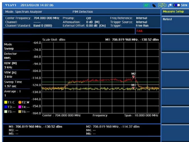
RF test — PIM Detection
